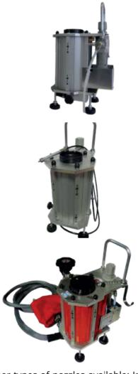
Other types of nozzles available: Int. Ø 1.5-2-2.5-3 L.115-3.5-4-4.5 mm cylindrical, and 2.5-2.5 L.115-4 L.115 mm Venturi with dry and **H20** guns; Int. Ø 2-3 mm selective, 2-3-4-5-6-8 Venturi with **HELIX** gun Blasting medium - air hose with protective sheath 3 m Abrasive material tank capacity: 2.5 l.
